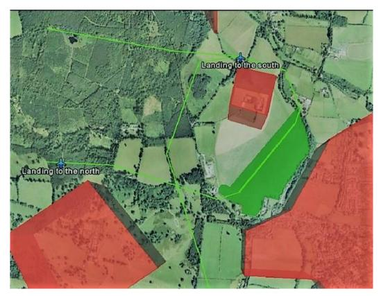
**Departures Runway 22**: After take off pilots must continue to track the extended centreline of the 'aerotow strip' for 0.5nm to avoid overflying properties on the airfield boundary and to the south of the airfield before turning on route. If departing to the west/ north west ensure the aircraft remains well to the south of Parham House.
